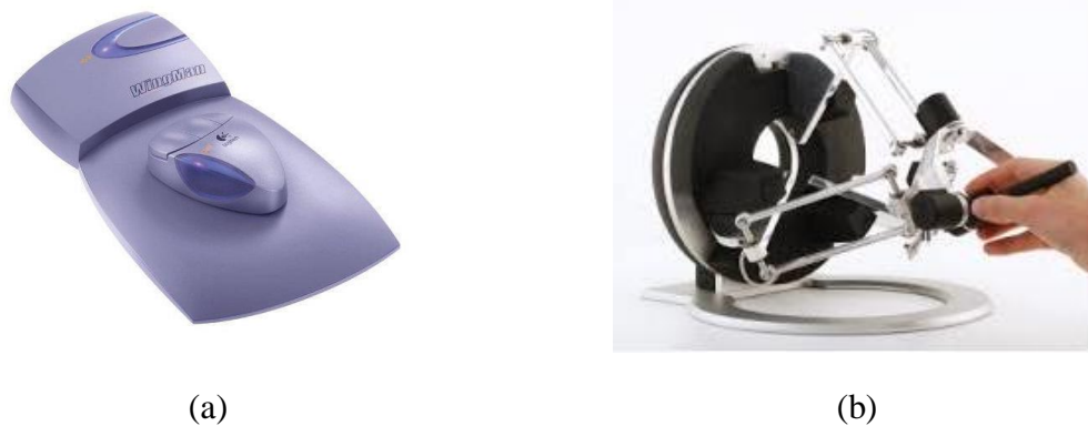
Figure 2.3 Examples of off-the-shelf haptic devices. (a) Logitech WingMan Force Feedback Mouse; (b) Force Dimension Omega 6.
