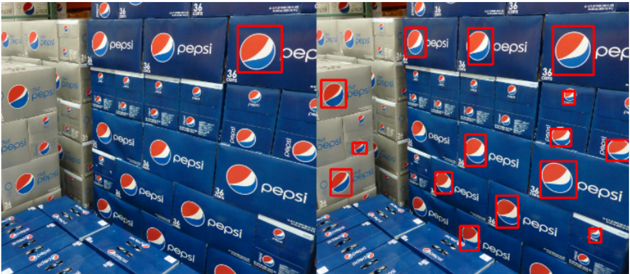
Figure 2.8. Small object detection to detect the company logo
