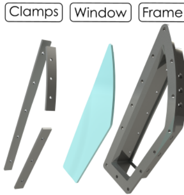
Figure 2.5: Window frame assembly exploded view
