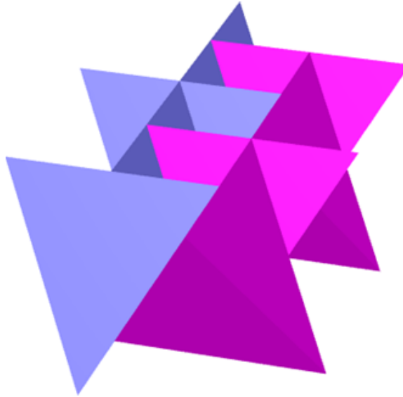
Figure 2.3. A general view of self-interlocking tetrahedra. Two column tetrahedra sections are displayed with different colors.
