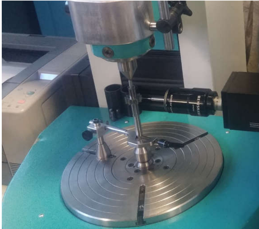
Figure 5.11. Measurement of conicity and concentricity errors on the gears with Wenzel WGT 350 gear metrology machine.
