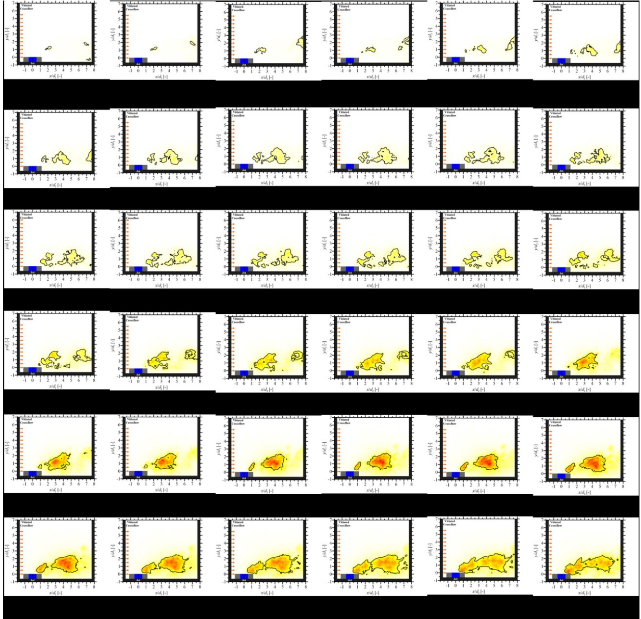
Figure 5.6: Ignition sequence using 50.4 kHz OH*-CL at Ma_\infty = 0.15 as \phi_j approaches 1.4.
