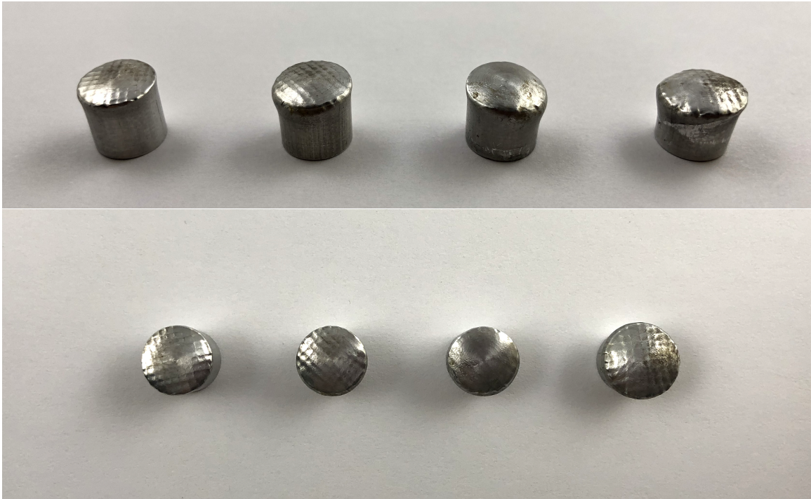
Figure 5.10. Photographs of (a) top and (b) elevated side profiles of post-impact 6061-T6 aluminum RCCs. Striking velocities of RCCs were (left to right) 364, 490, 561, and 601 m/s respectively. Progressively severe degrees of mushrooming deformation are shown with increasing striking velocities.
