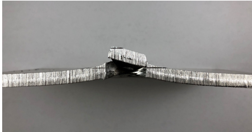
Figure 12.8. Side profile of nearly-ejected shear plug for a 6.35-mm thick plate. Plate exhibits severe bending. V_s = 165.4 m/s.
