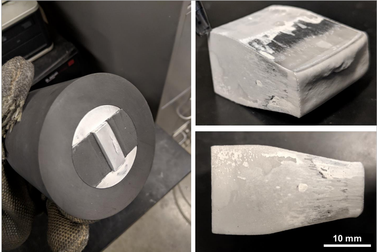
Figure 6.5. The alumina part after hot-extrusion.
