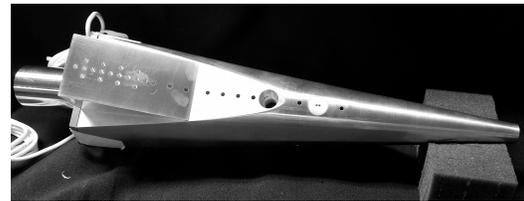
(c) Image of the long-ramp model with per-turber insert.
