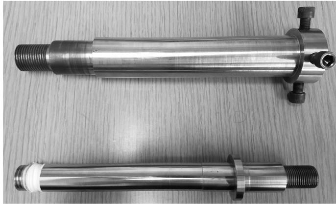
Figure 4.1. Image of the precision AoA adapter. The top piece is the outer sleeve and the bottom piece is the inner support.
