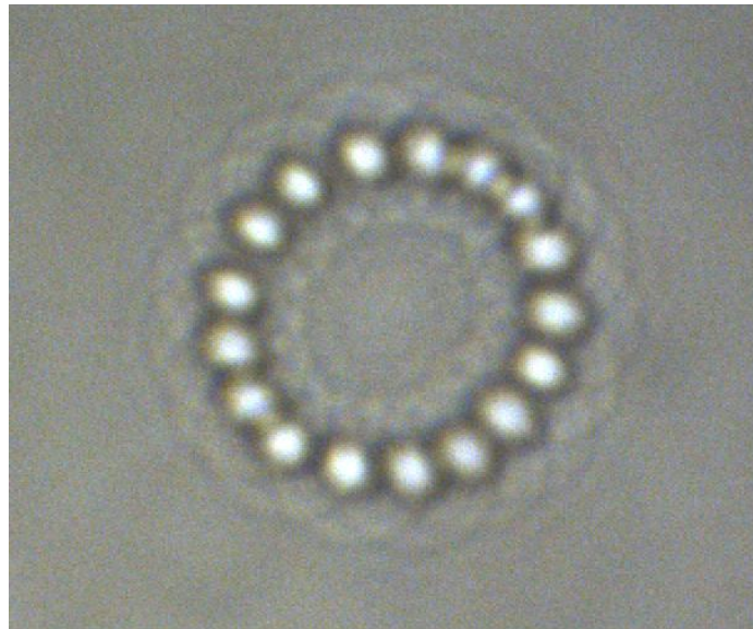
(b) Multiple silica microspheres (with diameter of 1.5 \mu m ) trapped inside a ring trap. The distortion is because of alignment imperfection of the imaging system.
