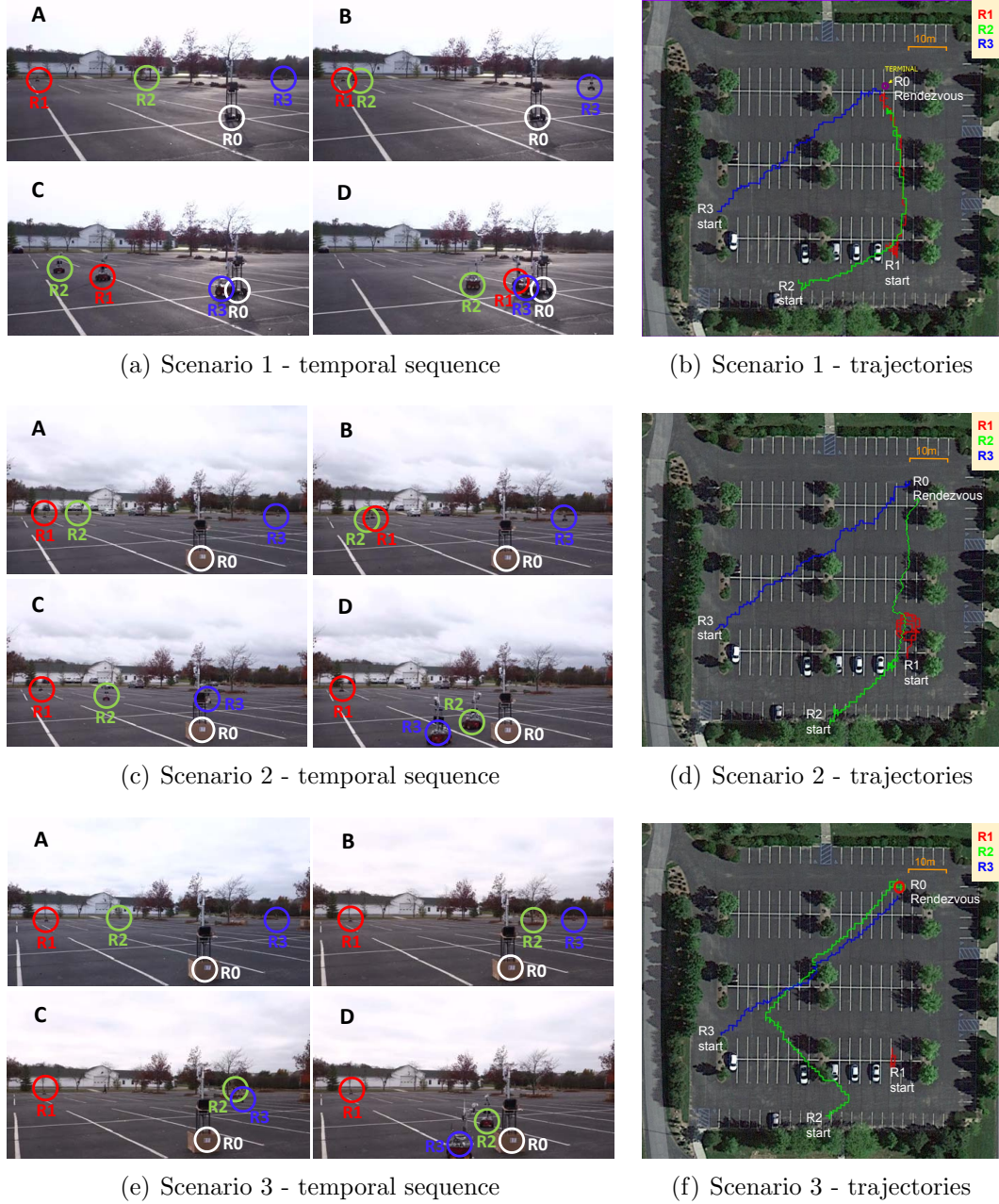
Figure 5.5. (a), (c), and (e) show a sequence of stills from experiments in Scenarios 1, 2, and 3. The temporal sequence is sorted alphabetically. (b), (d), and (e) are trajectories of the robots in Scenarios 1, 2, and 3 overlaid on the satellite image of the actual experimental site (a large and obstacle-filled parking lot). The trajectory of R_1 is depicted in red, the trajectory of R_2 is depicted in green, and the trajectory of R_3 is depicted in blue.
