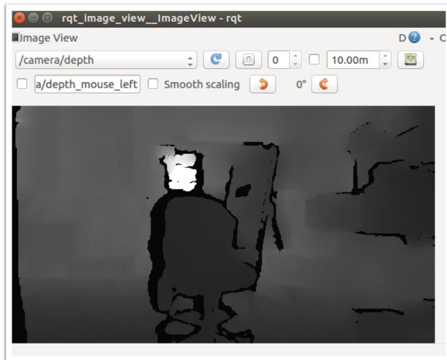
Figure 3.5. A example of a depth view from a stereo camera.
