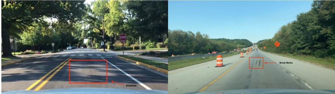
*Figure 2.1.* Example of noises in the road and lane detection.
