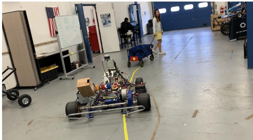
Figure 4.10. Using a cargo car as the leading vehicle to test ADTS.
