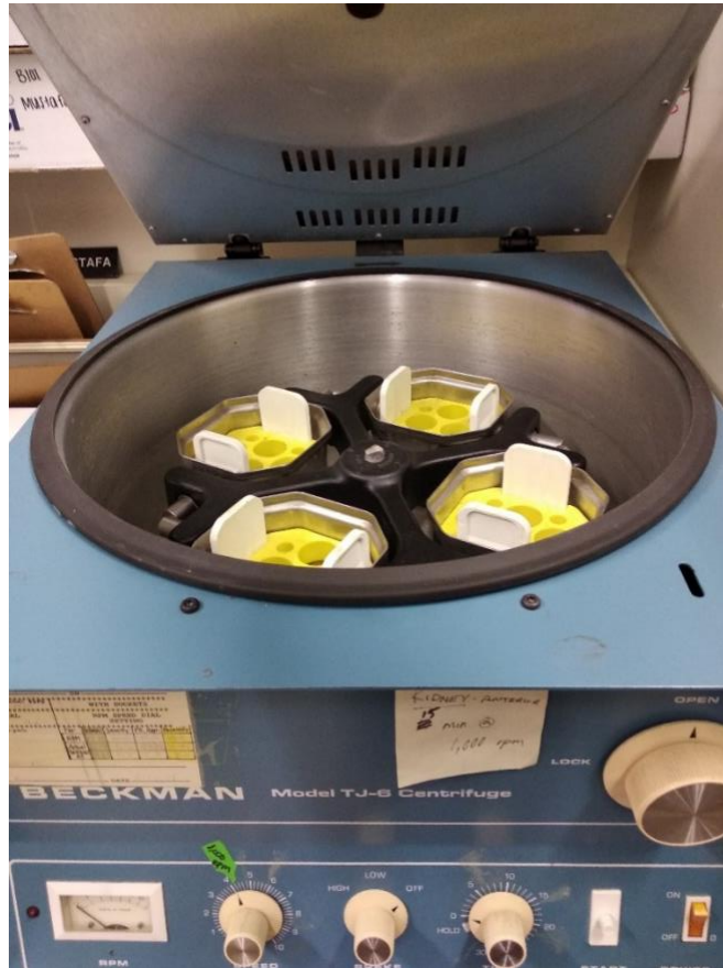
Figure 3.10. Centrifuge machine used for differentiating serum from blood.
