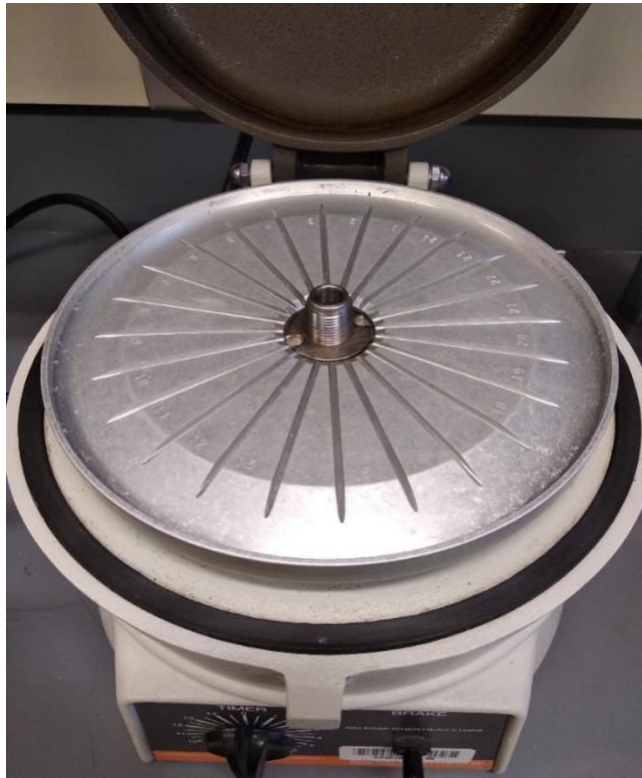
Figure 3.5. Centrifuge machine used for measuring PCV
