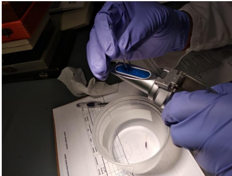
Figure 3.8. Measuring plasma protein using refractometer
