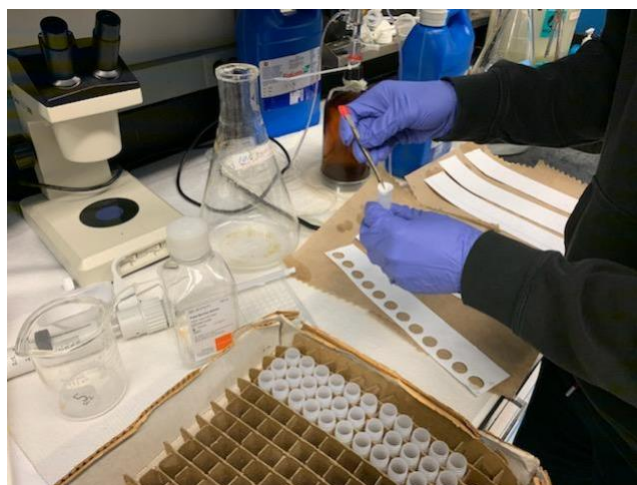
Figure 2.6. Transferring the filter paper in the scintillation vial
