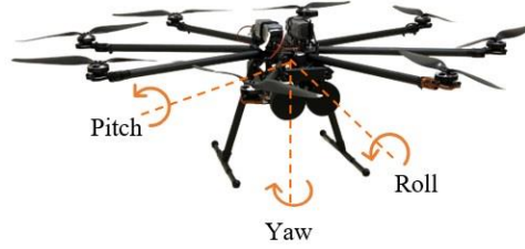
Figure 3.7. Rotations: Roll is the rotation around the front-to-back axis, Pitch is the turn about the side-to-side axis and Yaw is the direction of the heading of the UAV.
