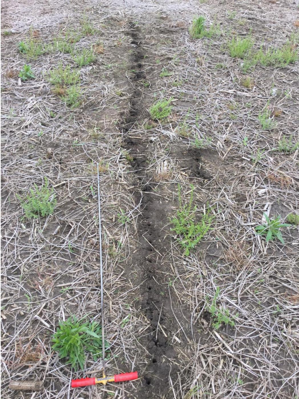
**Figure 5.4:** Tile probe and investigating the location of a tile line based on a specific probing interval (~7 cm).
