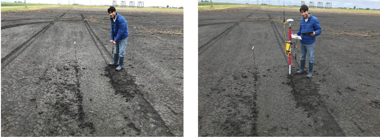
**Figure 5.5:** Probing to identify the locations of a tile line in the field (a) Once the first probe line located what appeared to be the tile line, the second probe line was used to confirm the identification. (b) Recording the confirmed location of a tile line with an RTK GNSS receiver.
