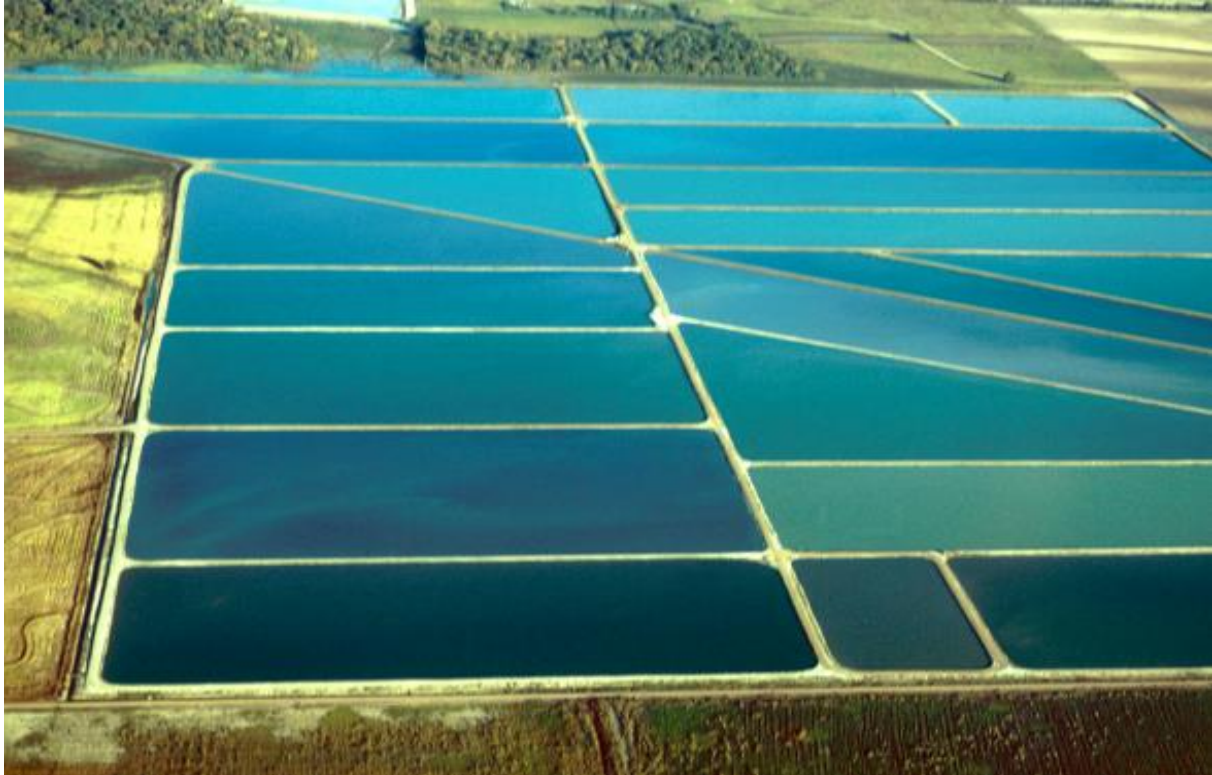
Figure 1.7. Semi-closed aquaculture system: levee pond (Avery, 2010)
