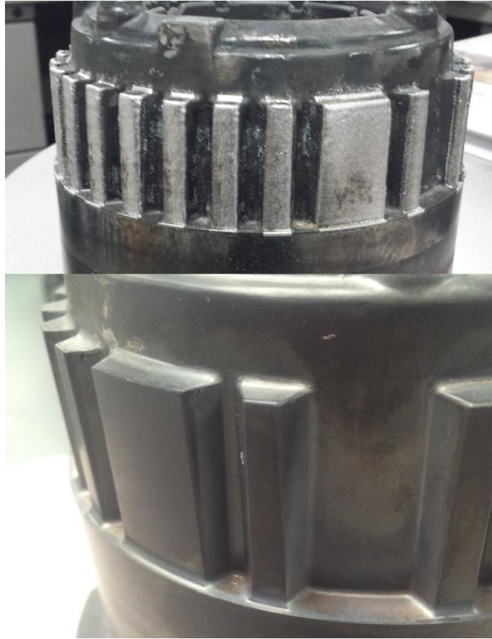
Figure 3.13: Industrial die insert after undergoing LDD to meet the requirements of a redesign before machining (top) and after machining (bottom).
