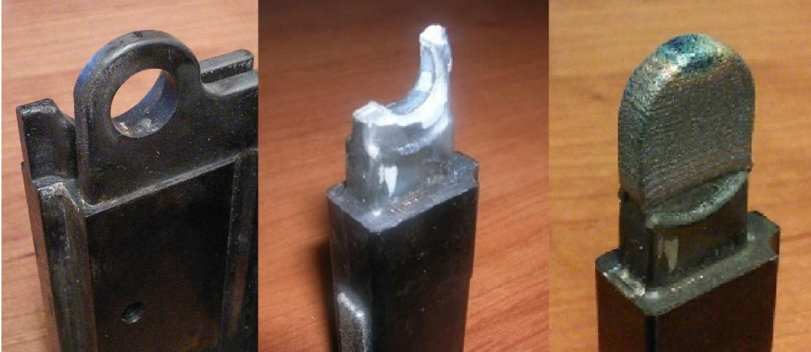
Figure 3.14: From left to right: unbroken insert with similar loop geometry, broken insert, and repaired insert. The repaired image was taken after LDD, but before machining and finishing.
