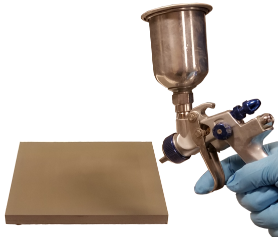
Figure 3.15. Liquid coating application with a high-volume & low-pressure (HVLP) spray gun.
