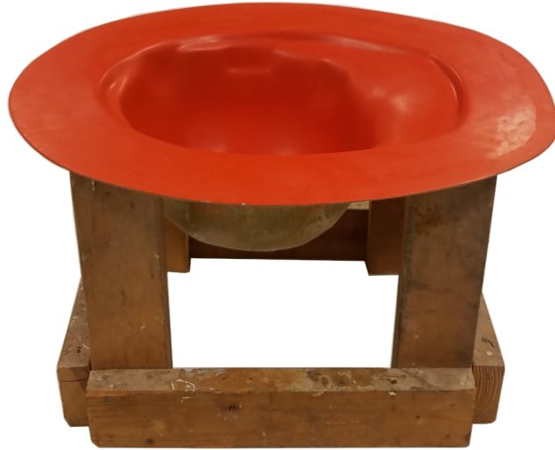
Figure 2.10. Fiberglass reinforced composite mold for composite part manufacturing.
