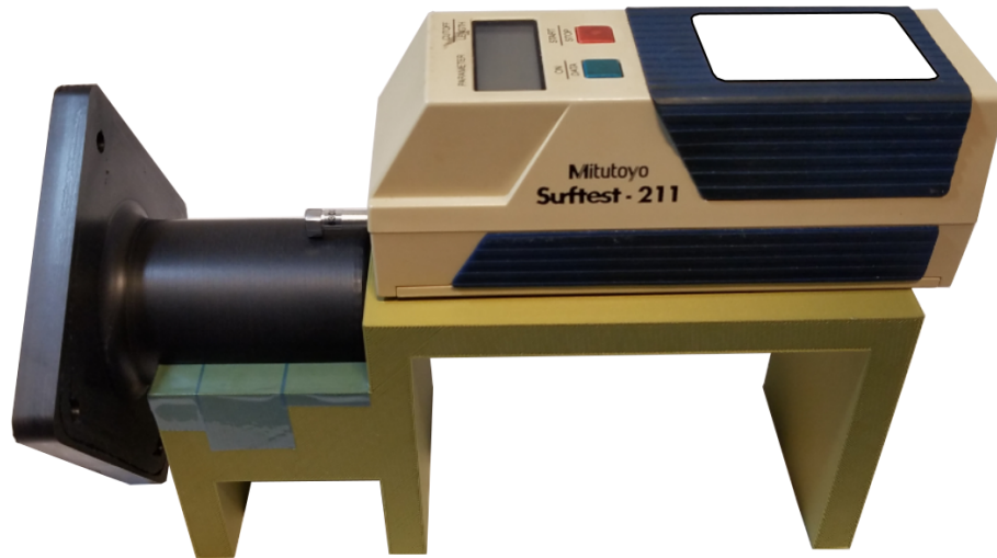
Figure 4.38. Roughness testing of the demolding test tool using the customized fixture.
