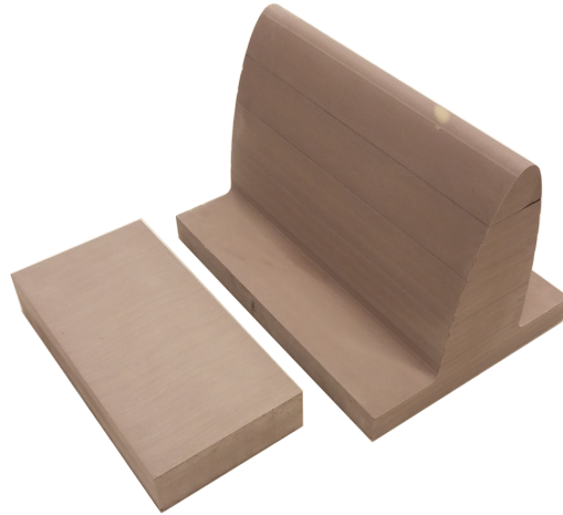
Figure 2.7. Tooling board composite part manufacturing mold.
