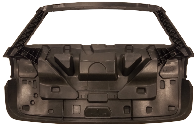
Figure 2.4. Sheet molding compound (SMC) composite liftgate for automobile.
