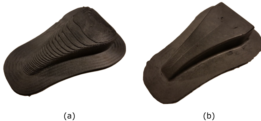
Figure 2.13. Additively manufactured composite mold (a) before and (b) after post-machining process.
