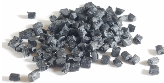
Figure 3.6. Pelletized carbon fiber reinforced polyphenylene sulfide (PPS) composite (50% carbon fiber by weight).
