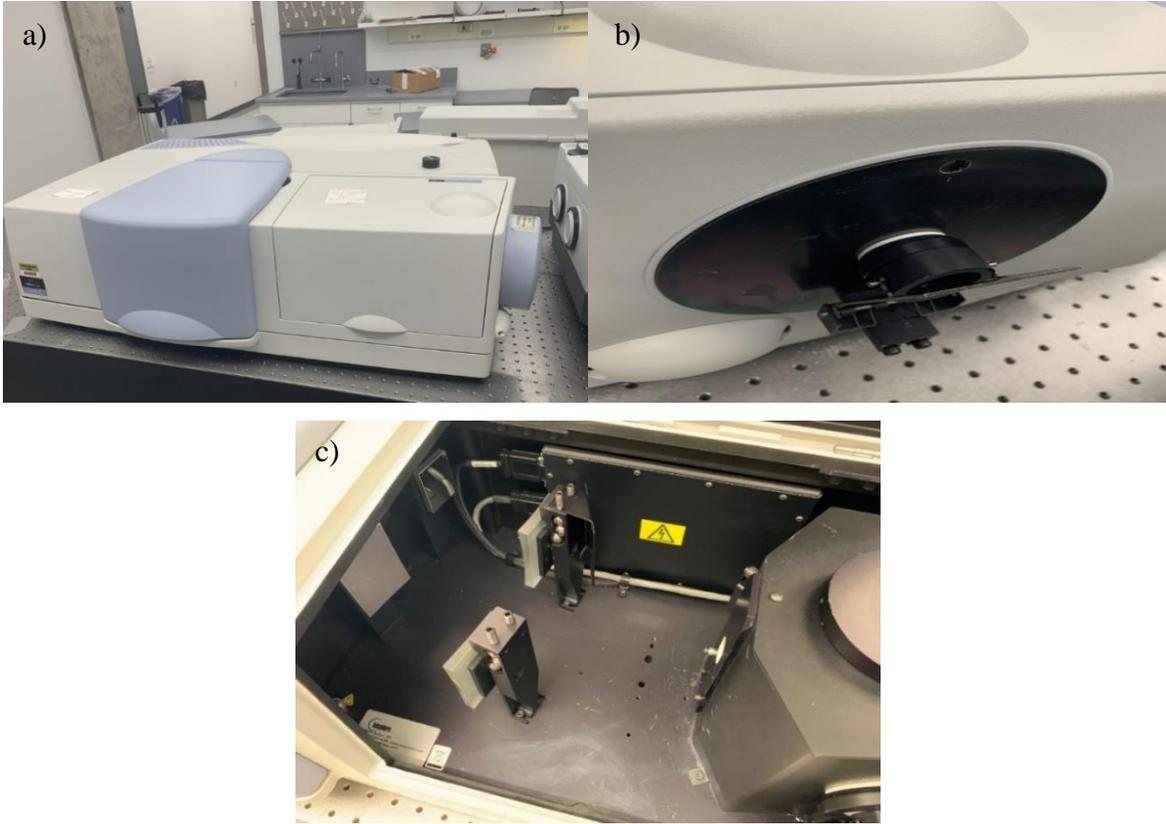
Figure 8. a) Spectrometer Lambda1050. b) The back. c) Inside
