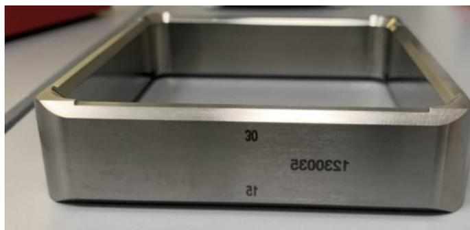
Figure 7. Tool used in controlling thickness
