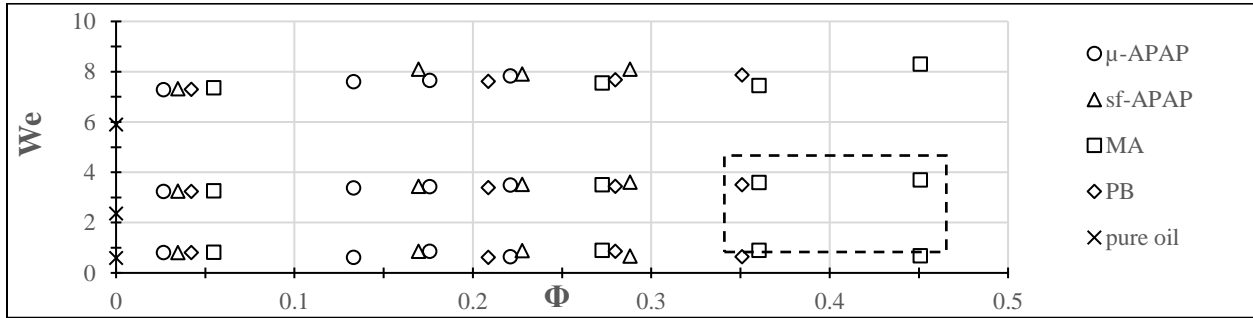
Figure 4.1. Printing of suspensions by Weber number and particle volume fraction, \Phi ; the dashed box contains suspensions that could not be printed reproducibly.
