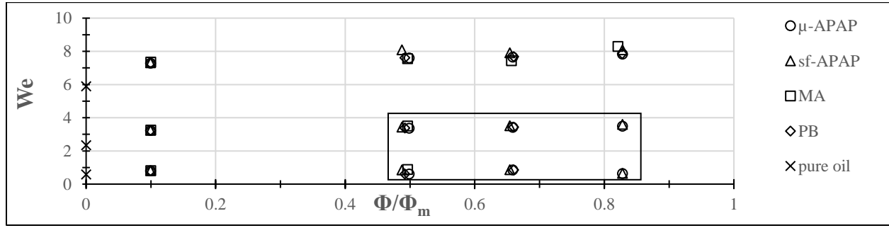
Figure 4.2. Feasible operating region, in solid box, based on the printing metrics for non-Brownian suspensions used in this study.
