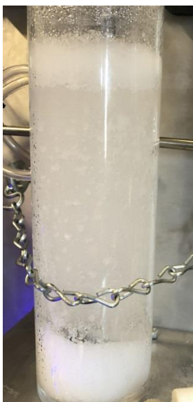
Figure 6.19. Reaction vessel following Test SBH-9. Solid particulate can be seen at the top and bottom of the reaction vessel.
