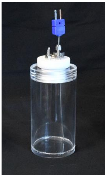
Figure 4.9. ABCharger 2.0 acrylic vessel.
