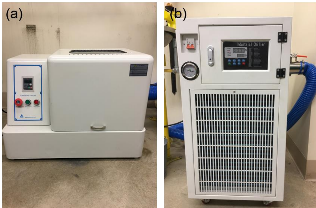
Figure 2.2. (a) Vertical high energy planetary ball mill and (b) chiller used in this thesis.
