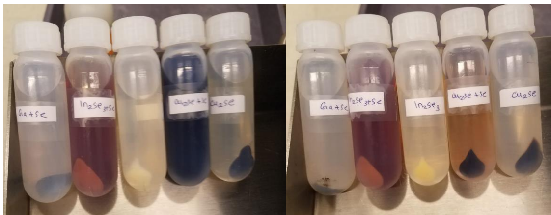
Figure 7.2. Antisolvent precipitation of various complexes one first and second purification cycles respectively.
