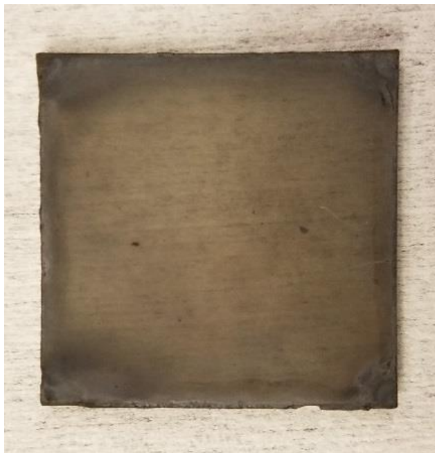
Figure A.6. Completed amine-thiol alternating layer CdTe film.
