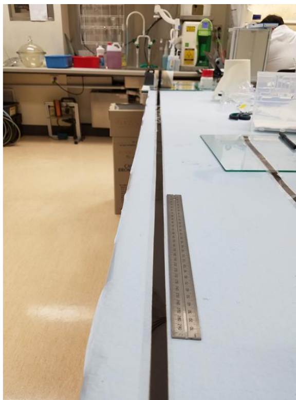
Figure 6.12. Roll-to-roll coater and section of CIGS nanoparticles coated from the optimized ink. The proof of concept roll-to-roll coating demonstrates the high uniformity over large lengths that the optimized ink and slot-die coater is able to provide.
