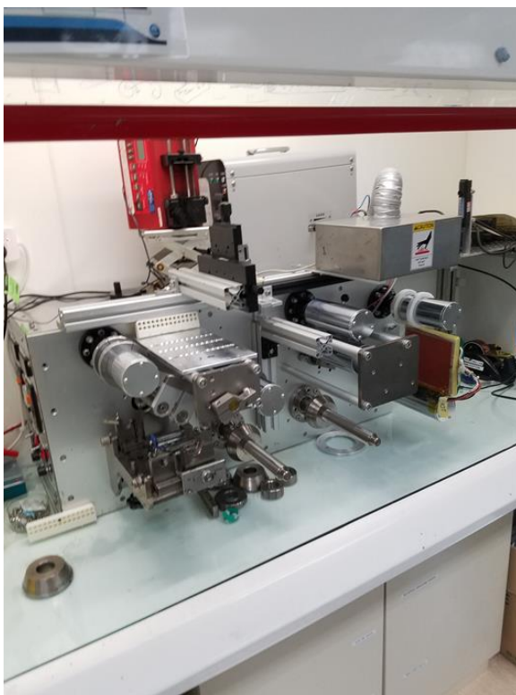
Figure 6.12. Roll-to-roll coater and section of CIGS nanoparticles coated from the optimized ink. The proof of concept roll-to-roll coating demonstrates the high uniformity over large lengths that the optimized ink and slot-die coater is able to provide.
