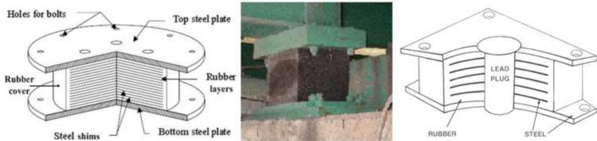
Figure 2-4. Schematic of Elastomeric Bearing (Left); Elastomeric Bearing On-Site (Middle); Schematic of Elastomeric Bearing with Lead-Core (Right) (Ealangi, 2010; Timothy et al., 2011; Choi, 2002)
