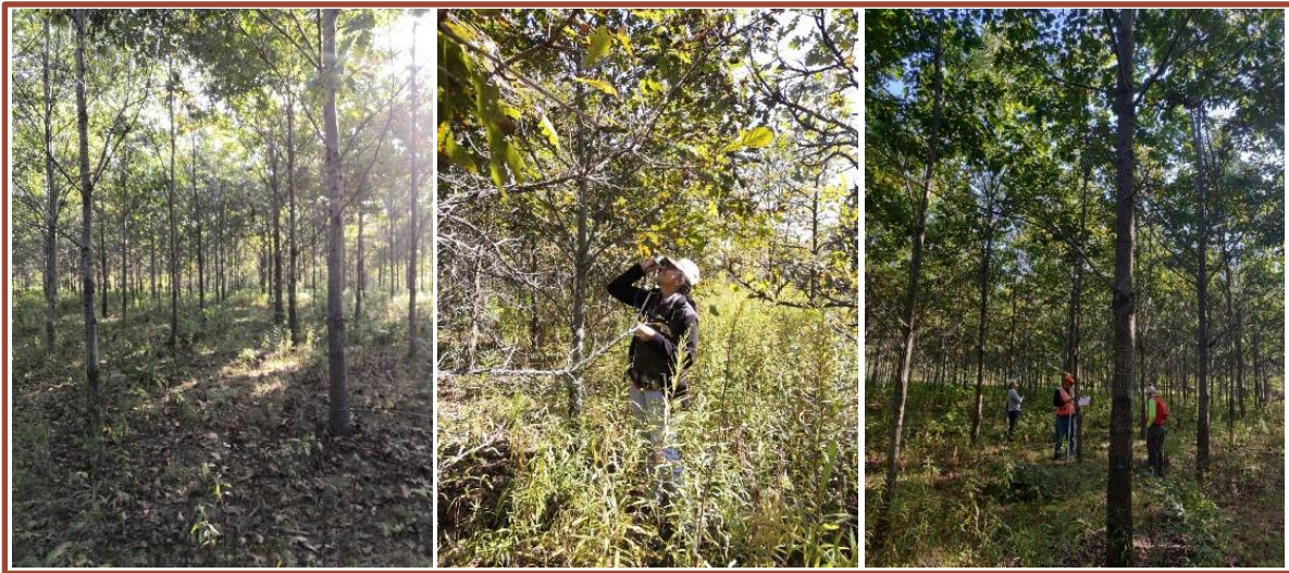
Figure 5. Ground measurements of tree height using Vertex IV hypsometer and crown diameter using a measuring tape.
