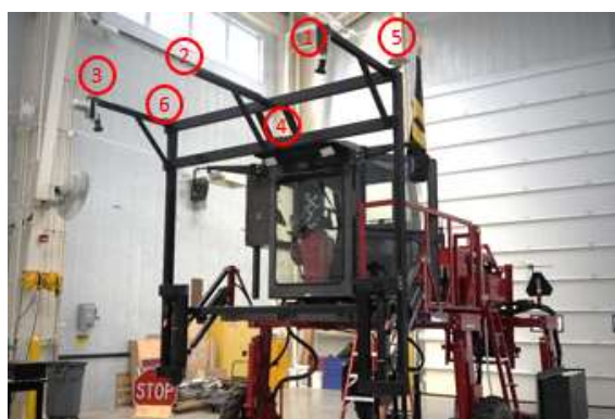
Figure 4.1. PhenoRover and the sensors on the platform including: (1) HDL-32E LiDAR, (2) Headwall MV, (3) HDL-32D LiDAR, (4) POS LV 125, (5) GNSS Antennas, (6) GNSS Antennas
