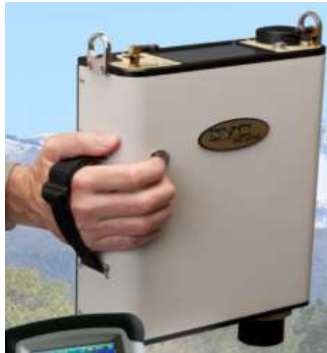
Figure 4.5. Spectroradiometer SVC HR-1024i (Spectra Vista Corporation) used for collecting the reflectance of ground targets.
