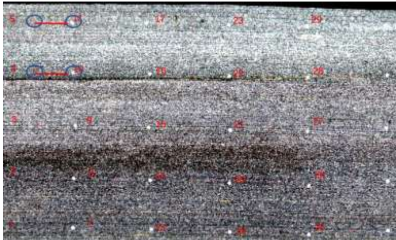
Figure 4.10. Image acquired for calibration after orthorectification by using different height values and mounting parameters: (a) mean of target heights and mounting parameters in Table 4.3, (b) mean DSM value and mounting parameters in Table 4.3, illustrating the stretch problem, (c) mean of target heights and mounting parameters in table 4.4, illustrating shift problem
