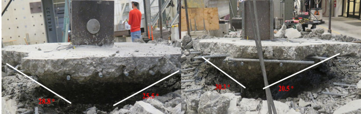
Figure 5.15 Breakout cone with average angle of 26.25 degrees
