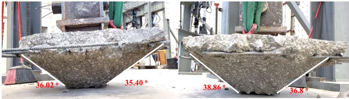
Figure 5.6 Breakout cone with an average angle of 36.77 degrees
