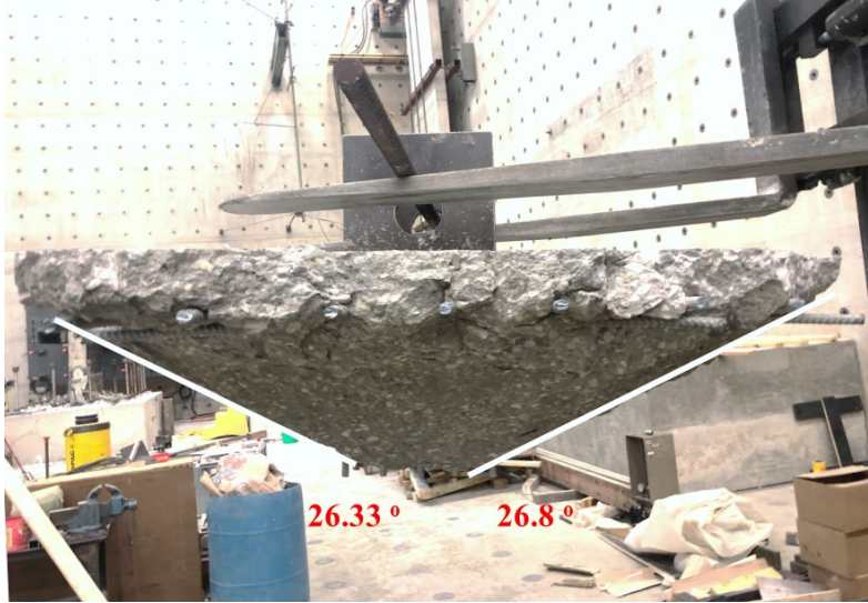
Figure 5.18 Breakout cone with an average angle of 26.56 degrees
