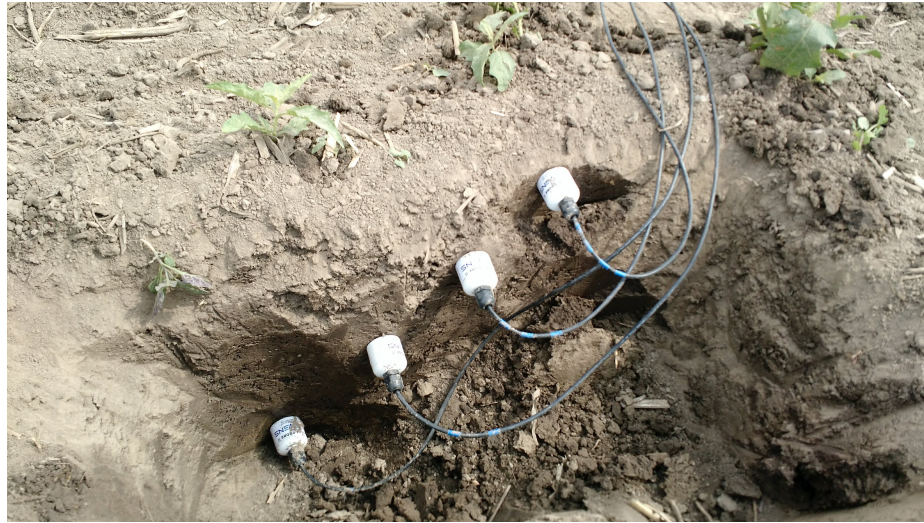
Figure 1.2. The HydraProbes used for in-situ measurements for tower experiment 2018 [10]
