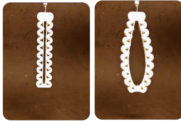
Figure 50. Bending-open behavior under a pressure of 25 psi.
