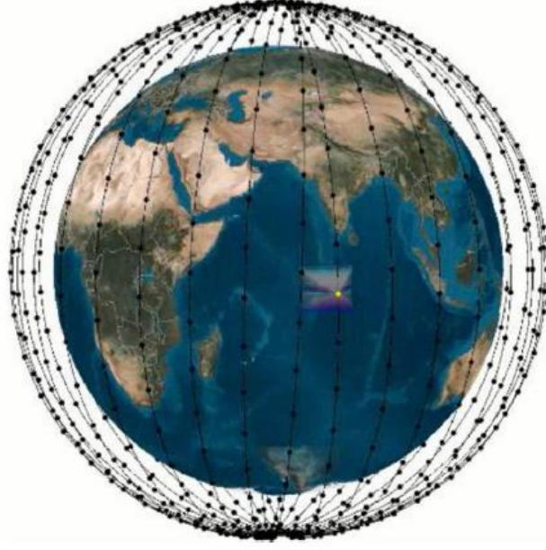
Figure 2.2: One Web’s polar constellation design using an 87.9^\circ inclination, viewed from the equatorial plane (del Portillo et al., 2019)
