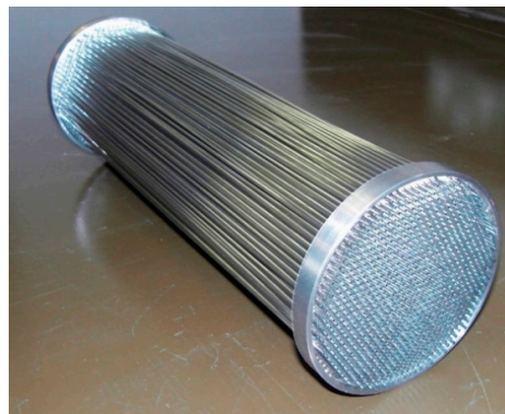
Figure 8. Heat exchanger core of ammonia/carbon heat pump generator [35].
