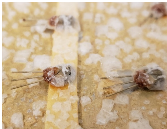
Figure 5.14. Salt crystal formed after a water evaporated in salt water experiment.
