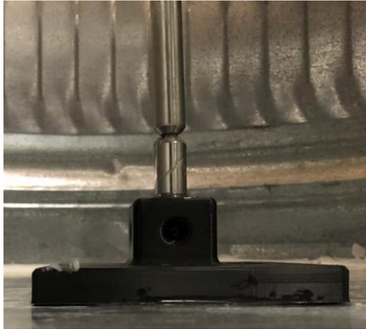
*Figure 3.4* Image of the bottom support.
