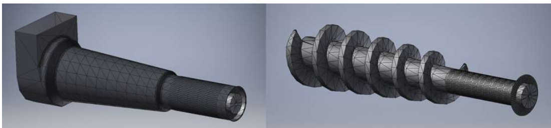
Figure 4.7: The meshed surface of the screw. The mesh properties were chosen to avoid long, thin elements which adversely affect the way boundary forces are calculated within DEM.
