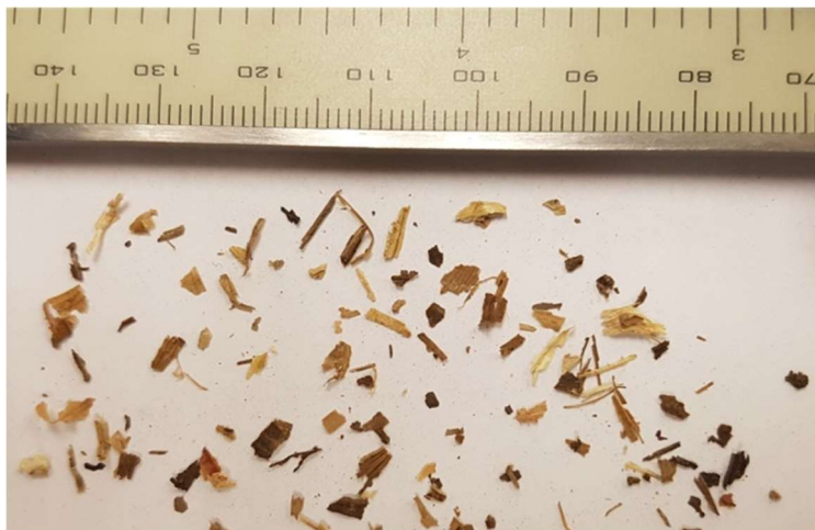
Figure 4.10: Corn stover shape and size with a ruler for scale. The particles are mostly plate-like, with millimeter scale dimensions in two directions and tenths of millimeter dimensions in the third direction. Other particle shapes include narrow, rod-like particles with only a single dimension on the scale of millimeters, and brick-like particles with all three dimensions on the millimeter scale.
