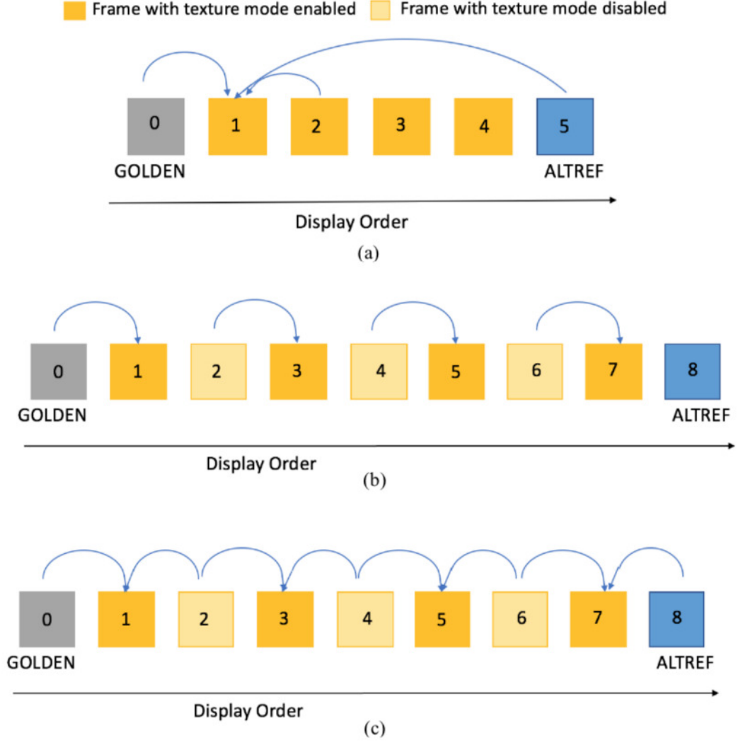
Fig. 4.6.: Coding structure of texture mode: (a) GF Group Coding Structure Using tex-all Configuration. (b) GF Group Coding Structure Using tex-sp Configuration. (c) GF Group Coding Structure Using tex-cp Configuration.
