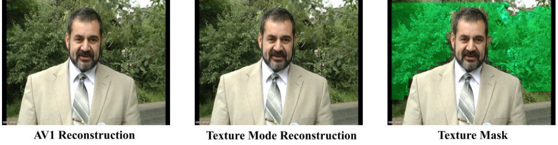
Fig. 4.13.: Visual comparison of a sample reconstructed frame using AV1 baseline and our proposed texture mode, along with the texture mask used.
