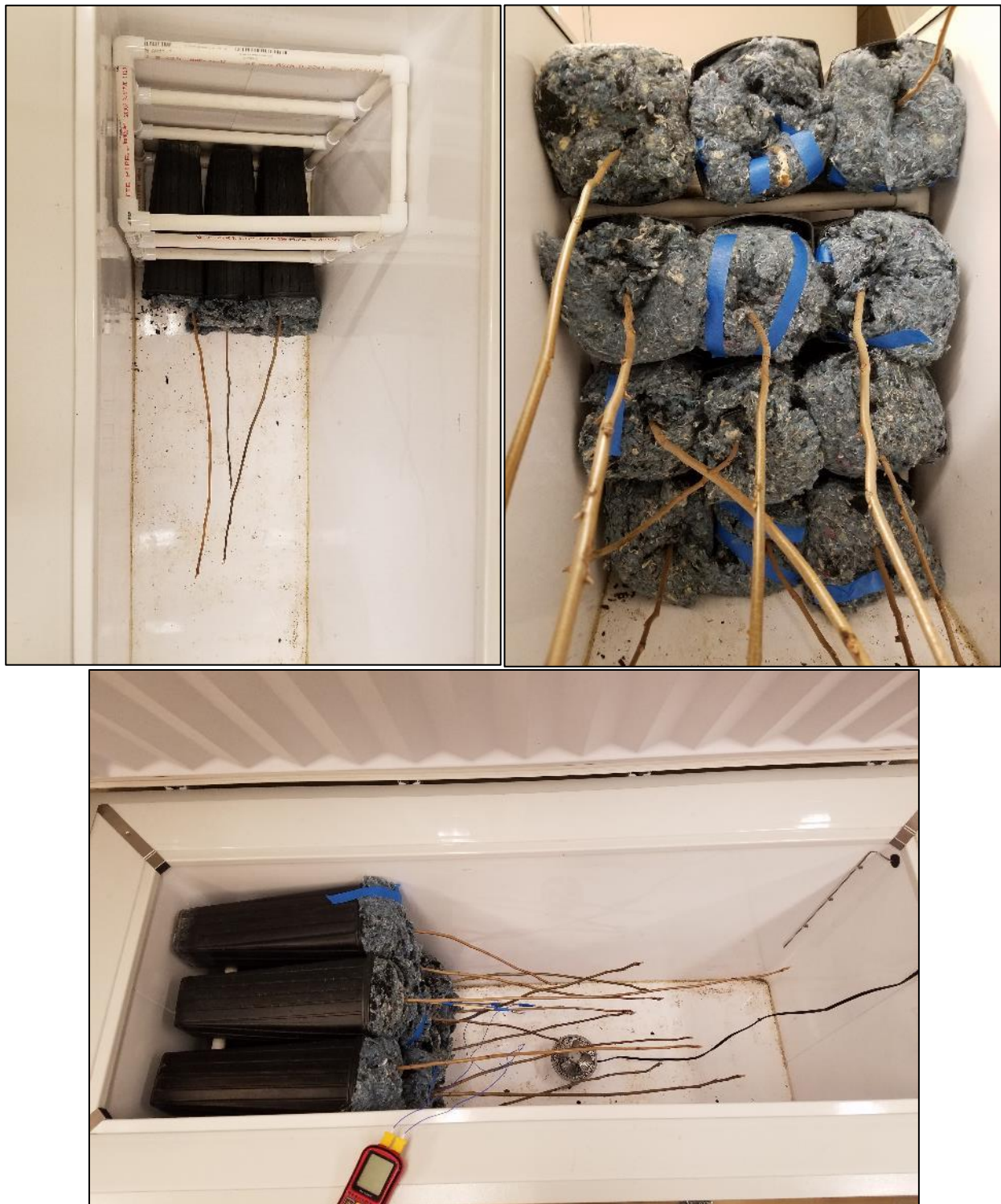
Figure H.30. For the freeze treatments, seedlings were placed on a custom-made PVC pipe rack (constructed with help from James Warren) inside a programmable freezer with a small fan to evenly distribute air temperatures, along with numerous soil and air thermocouples and data loggers to monitor temperatures.
