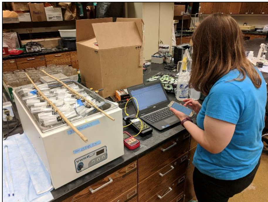
Figure H.12. When the hot water bath reached the target temperature, two sample poles were suspended over the bath. The temperature of the sample and water thermocouples was recorded every 5 minutes.
