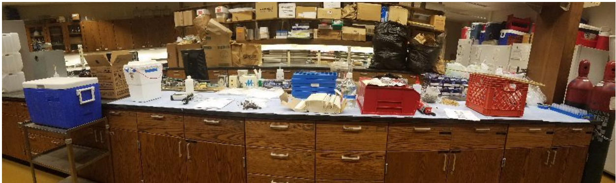
Figure H.8. Laboratory bench set-up for heat test from left to right: sample coolers, fluorimeter, leaflet prep areas, sample pole mounts, and post-batch sample processing.
