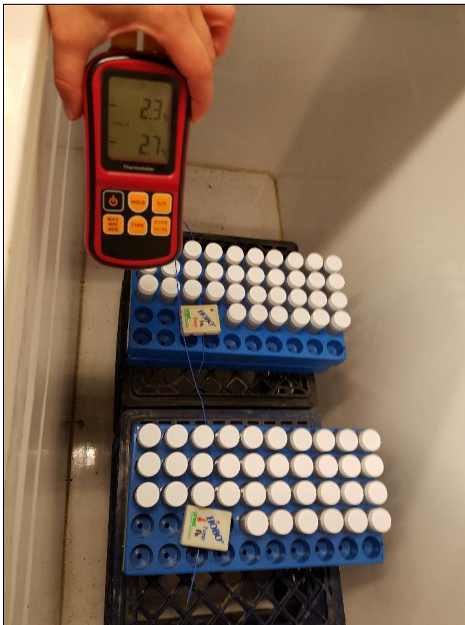
Figure H.19. Prepared samples were then placed into a pre-chilled programmable freezer with thermocouples and data loggers to receive cold treatments.
