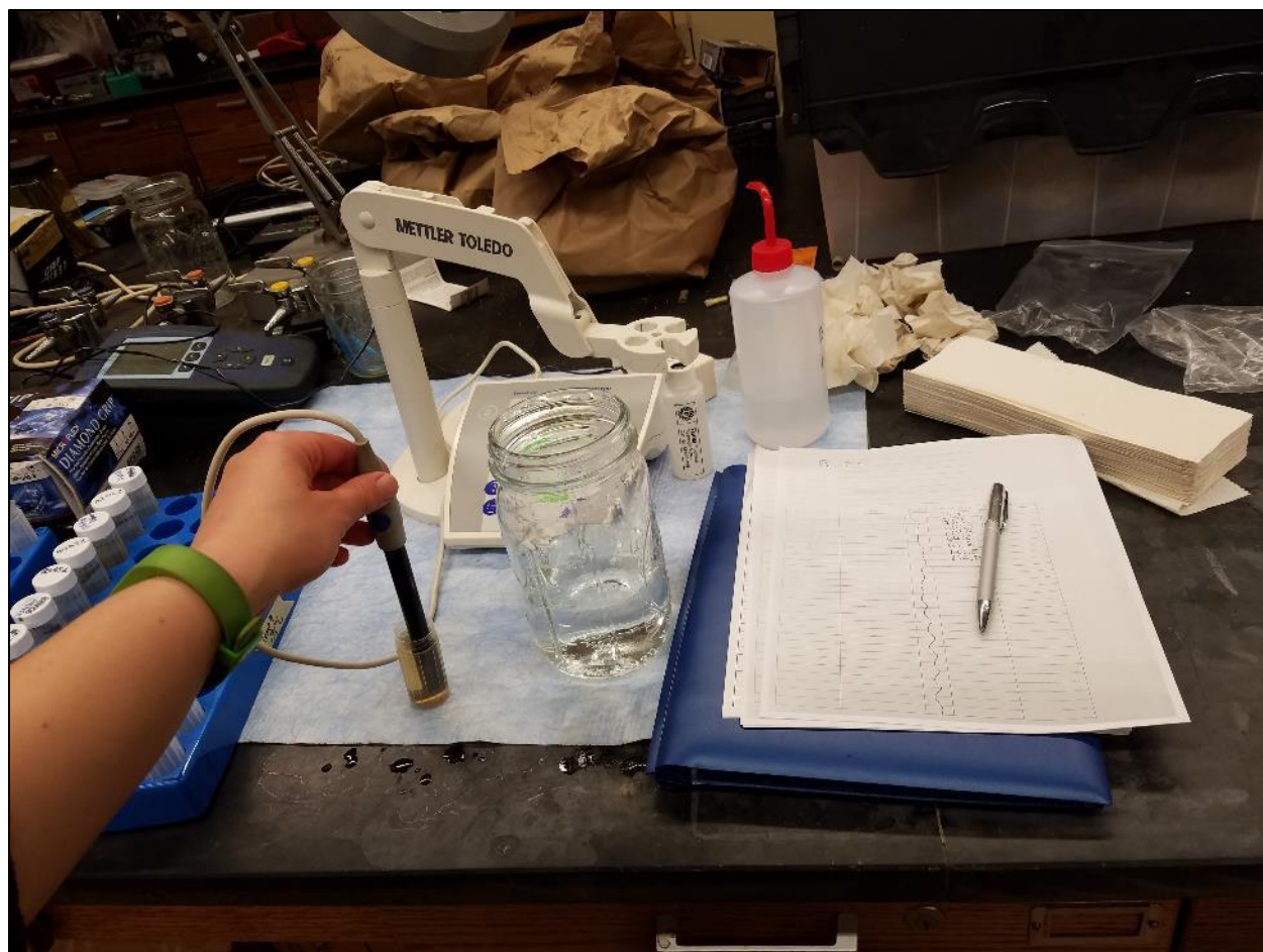
Figure H.20. Electrolyte leakage (EL) into the water was assessed using a conductivity meter after complete thaw and again following autoclaving to induce 100% EL.
