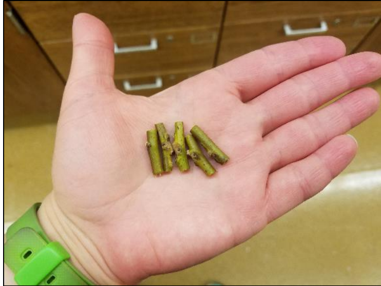
Figure H.17. Twig samples were cut into five 1-in. segments, one for each cold treatment.
