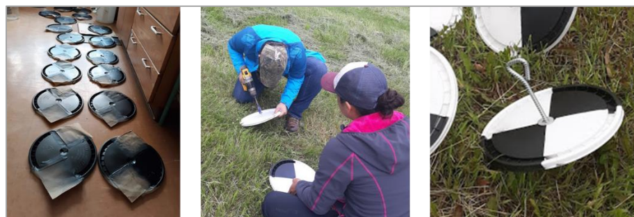
Figure 2.1. Ground Control Points (GCP) installed at PPAC, TPAC, ACRE and Simpson, and used for coregistration of images between flights.
