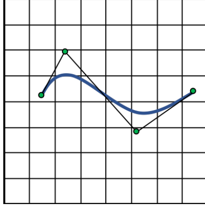
Figure 1.3. : Schematic of enriched isogeometric analysis containing an explicit interface immersed in a non-conforming mesh. Both the explicit interface and the underlying domain contribute to the behavioral field solution.
