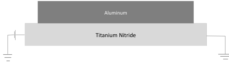
Figure 2.4. : Schematic of the Blech-structure that was used in the simulation.
