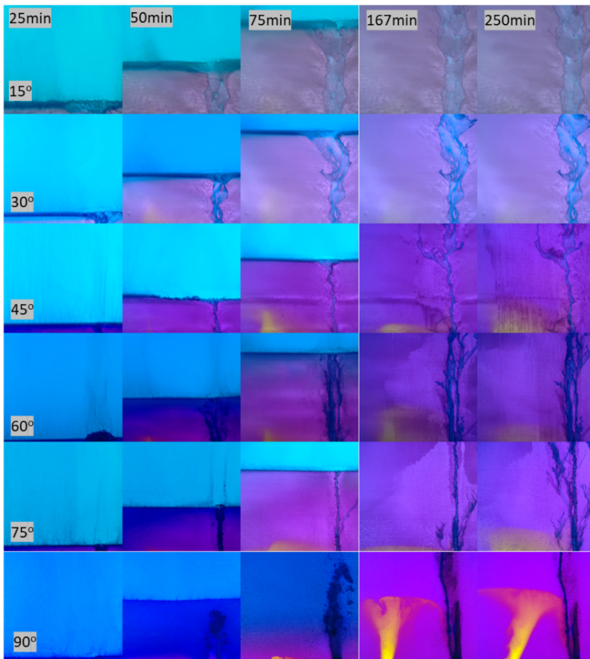
Figure 3.10 Images of reactive miscible fluids mixing with different angles of inclination at time T=25, 50, 75, 167, 250 minutes. Aperture is 2 mm; pumping rate is 0.17 ml/min for both Solution 1 and 2; density contrast is 1111/1031.8
