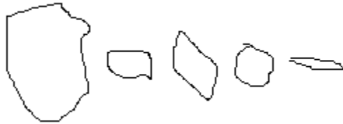
Figure 5.2 – Examples of the varying cross-sections that could be found in a copper sulfide concentrate (after Perrez-Tello et al. [16] and [99])
