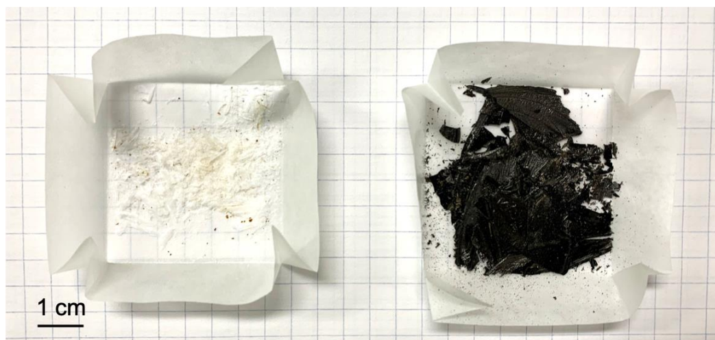
Figure 3.16. Optical images of silica sol-gel coated wing scales after firing in air (left) and in inert Ar atmosphere (right).
