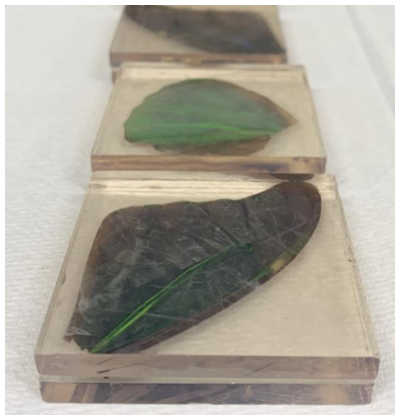
Figure 3.2. A photograph of SiO 2 coated M. rhetenor wings clamped between two glass substrates.
