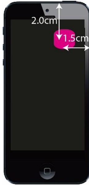
Figure 42. Position of magnetic sensor in iPhone 6 [110]
