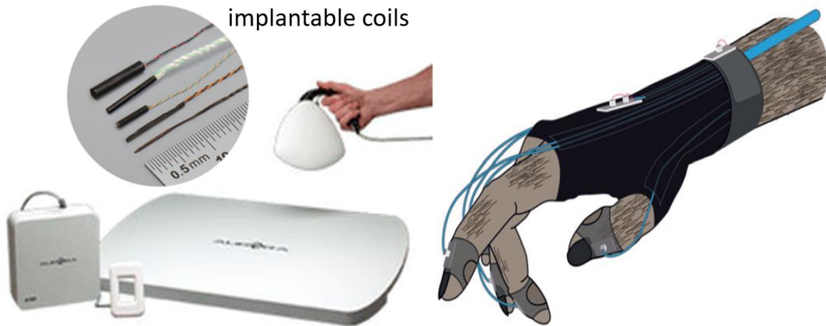
Figure 5. Some applications of magnetic tracking system. Left: NDI Aurora magnetic tracking system capable of tracking catheters and biopsy needles, insight shows the implantable magnetic sensors (coils); right: wired magnetic tracking system for hand motion tracking.
