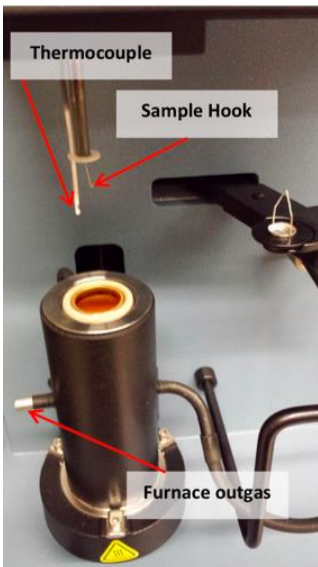
Figure 26. Thermogravimetric analyzer furnace setup.
