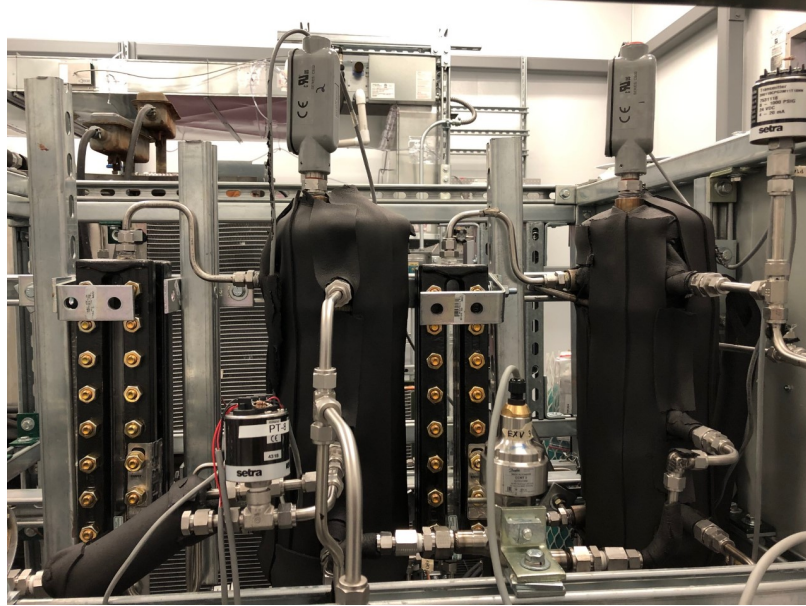
Fig. 2.7. Photo of liquid level measurements in the CO 2 test stand.
