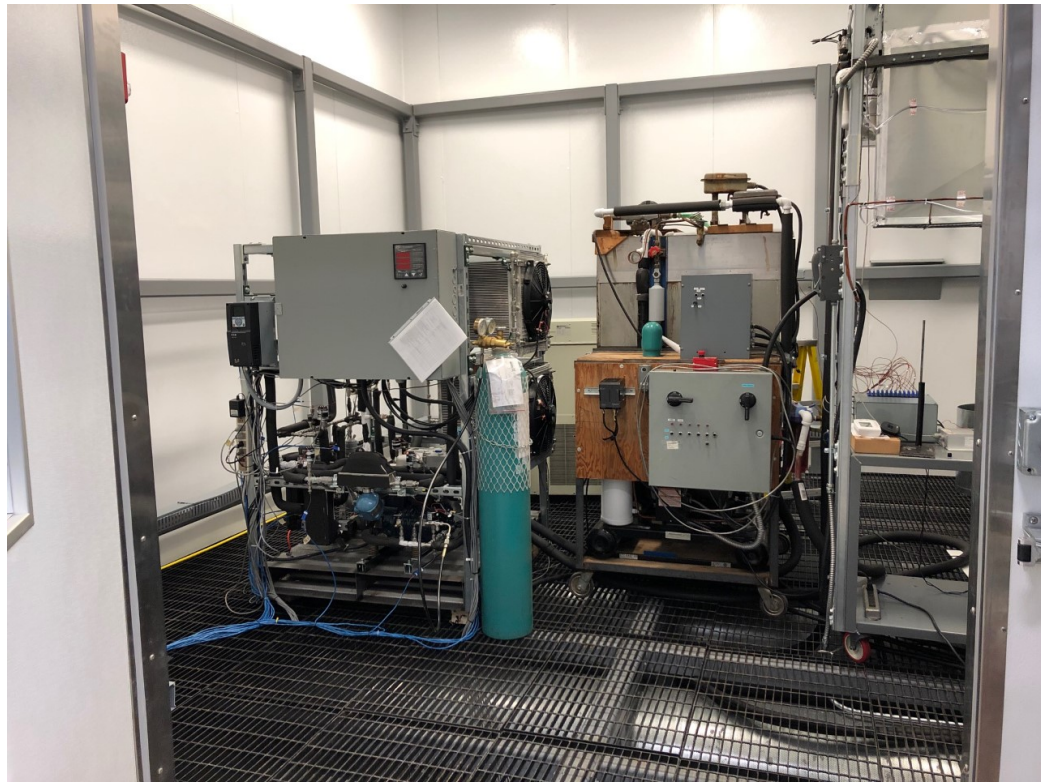
Fig. 2.1. Photo of the completed transcritical CO 2 test stand inside of a psychrometric chamber.
