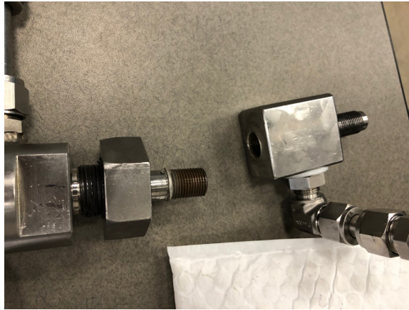
Fig. 3.12. CO 2 ejector with broken solder joint and galled threads.
