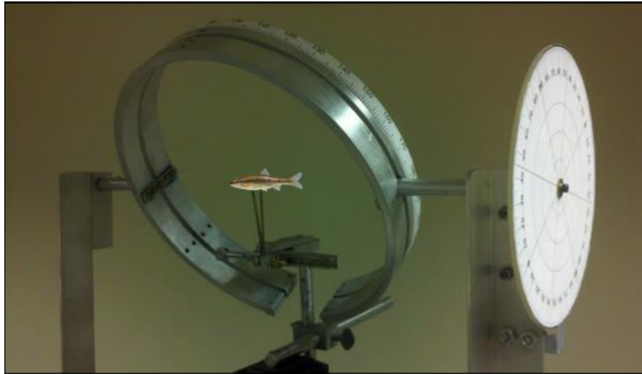
Figure B2. Closeup of the apparatus with fish model in view. For accurate measurement, the fish is placed in the center of the apparatus where the head and body are aligned in the horizontal plane, 90^{\circ} - 270^{\circ} . The circular rotating metal arm has angular coordinates along the outer perimeter, used for determining the width of the visual field along various elevations around the head.
