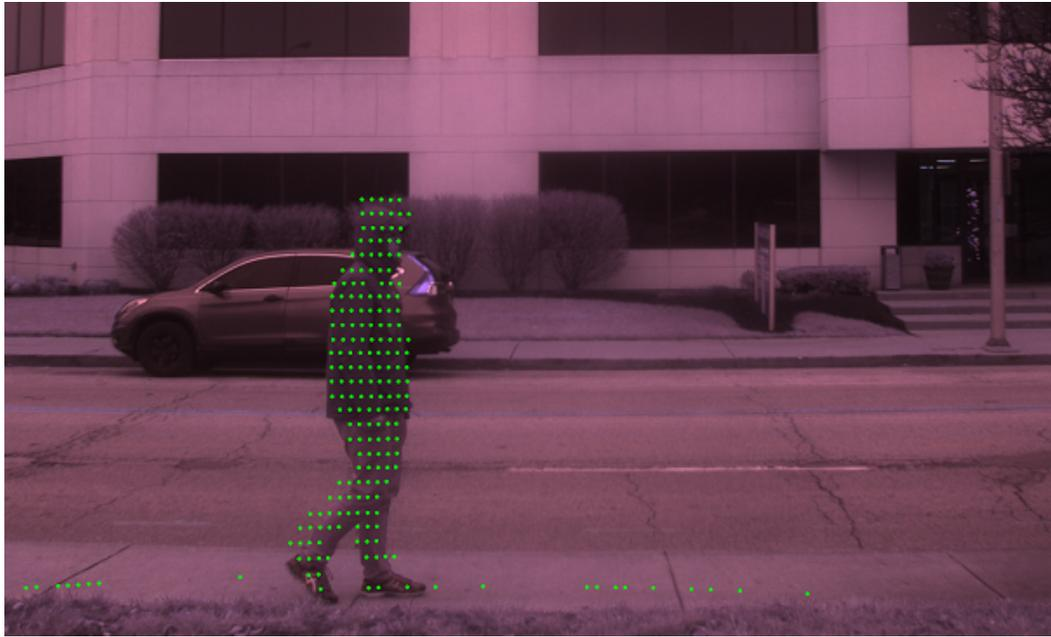
Fig. 4.8. Overlay showing fusion on data with LIDAR points filtered to allow points only within a distance (LIDAR Horizontal Resolution = 1024)
