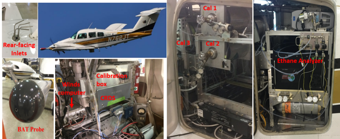
Figure 2.1. Purdue's Airborne Laboratory for Atmospheric Research (ALAR) with specific instruments labelled. The roof inlets are used rather than the large front-facing inlets as there was some evidence of leaking air in the large manifold.
