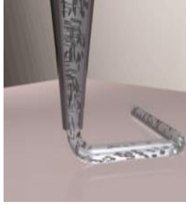
Figure 3.12 Schematic showing the extrusion of Te/PDMS composite from nozzle and shear-force induced alignment process.
