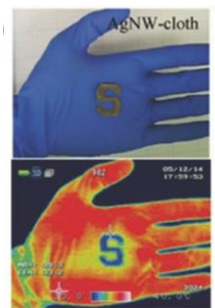
Figure 1.7 Thermal images under IR camera for the S-shaped Ag nanowires cloth 23 .
