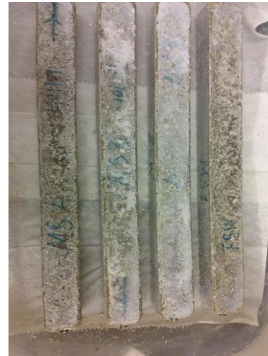
Figure 2.3. Appearance of the mortar bars exposed to magnesium sulfate (MS): left – SC mortar bars after 18 months of exposure; right – OPC mortar bars after ~9 months of exposure
