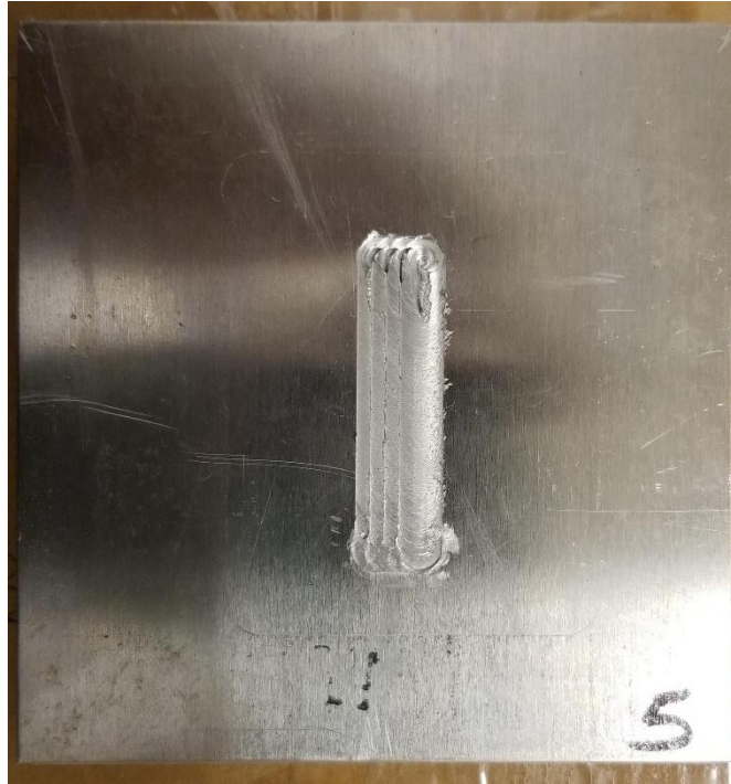
Figure 2-4: The top view of the weld adding 5 plates on the substrate.
