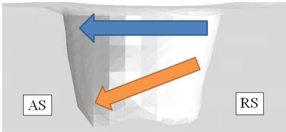
Figure 4-1: Sound weld cross-section (at the center of the model). (Top left pointing blue arrow-shoulder-driven flow; down left pointing orange arrow- pin-driven flow).
