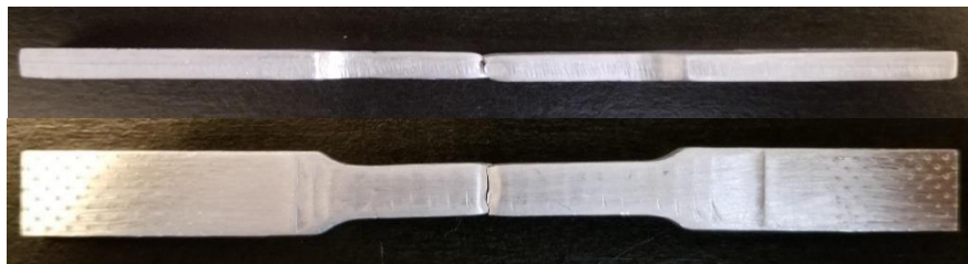
Figure 4-21: Tested FSAM processed sample after fracture .
