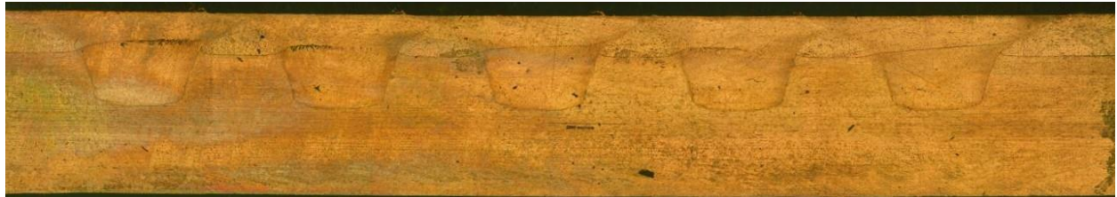
Figure 4-31: Macrostructure of the addition of 1 mm plate to a 3.17 mm plate.
