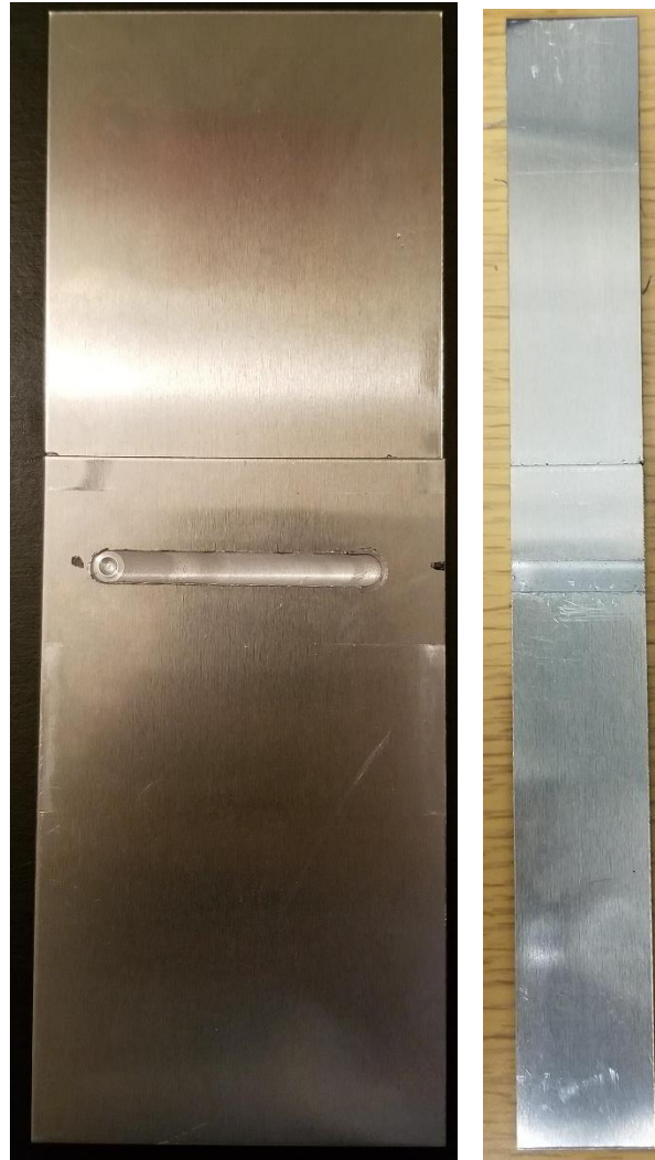
Figure 4-23: Friction Stir lap weld sample and Tensile shear test specimen..
